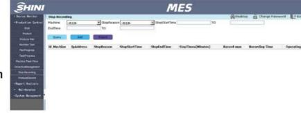
through two ways: (1) directly chosen in software; (2) when man-made shutdown happens, the system will generate a record, including time and cause, both of which will be matched with that automatically collected in the shutdown record of IMM's, and ultimately the cause of shutdown will be automatically transferred to the records in IMM.
